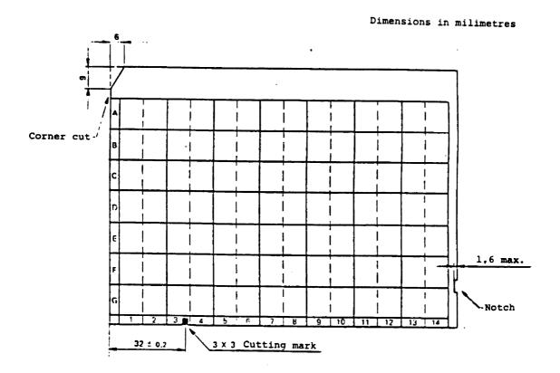
Figure 3 – Example of microfiche of uniform division, using image arrangement No. 2
